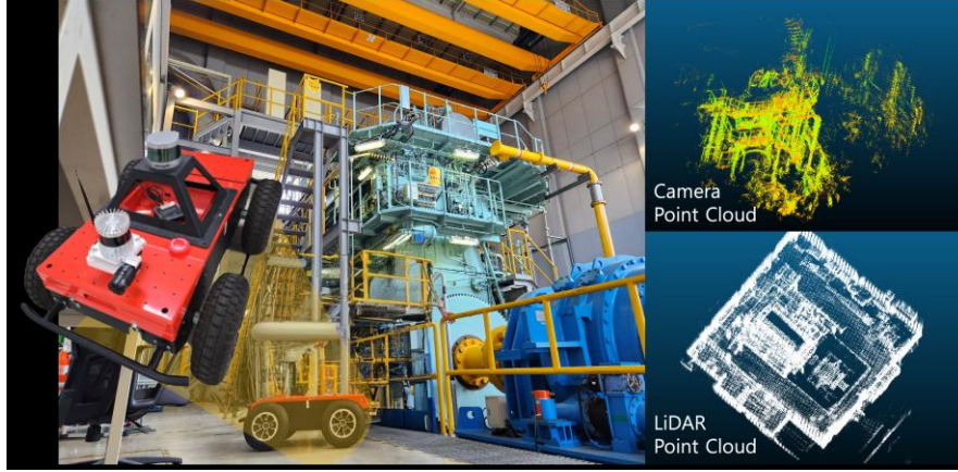
Fig. 2. Rover and environment used for dataset generation
