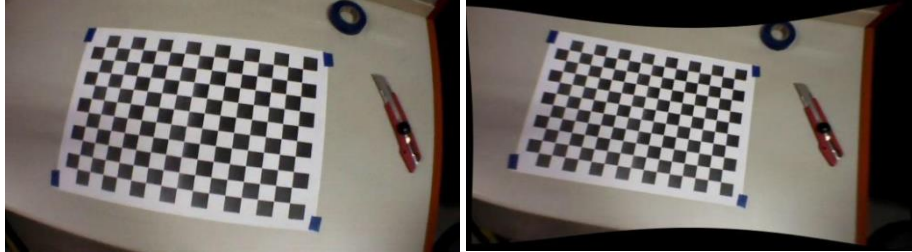
Fig. 3. Before and After Image of the Undistortion Operation (Left: Before, Right: After)
