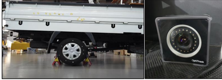
Fig. 3. Experimental setup with motion capture system
